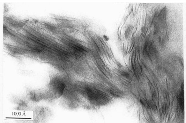
Figure 2. TEM image of an epoxy-clay composite containing 20 wt % \text{CH}_3(\text{CH}_2)_{17}\text{NH}_3^+ -montmorillonite.
